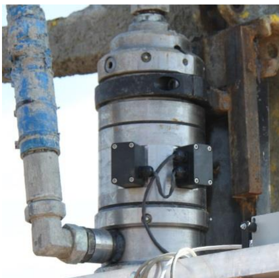
Figure 9 Interface at the flushing head
