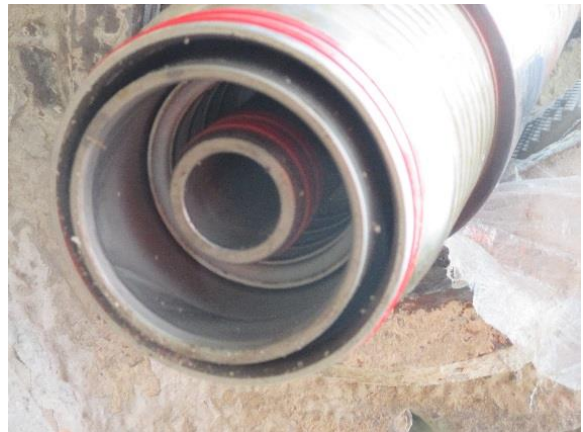
Figure 3 Multi-channel drilling rod .
