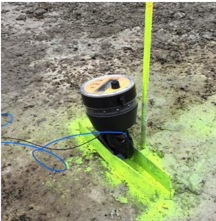
Figure 12: Data logger on the acceleration cone
