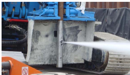
Figure 1: Jet grouting beam
